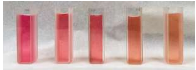
Figure 5. Mixture solution for 0.01 mol of Beetroot solution with copper solution (from right : 200 ppm, 100 ppm, 50 ppm, 25 ppm, and 12.5 ppm)
